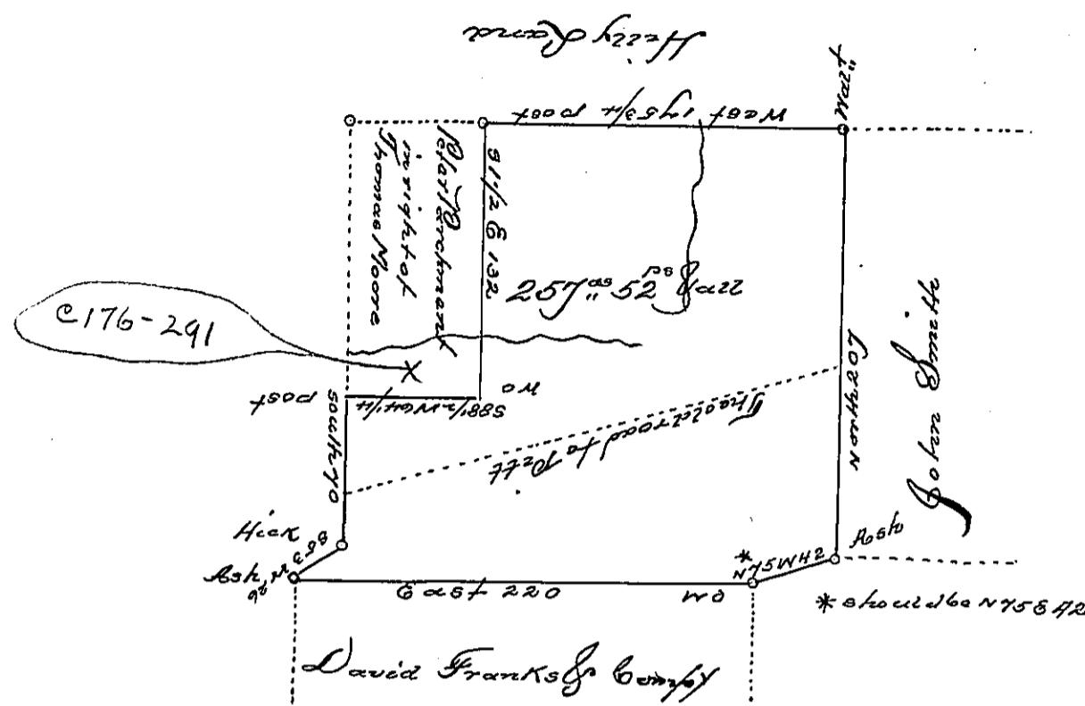
A Draft of a tract of Land containing 359<sup>1</sup>/<sub>2</sub> ac 52<sup>1</sup>/<sub>2</sub> sq. allowance being part of a larger tract of land containing 309<sup>1</sup>/<sub>2</sub> ac 52<sup>1</sup>/<sub>2</sub> sq. Surveyed by Robert McCrea
